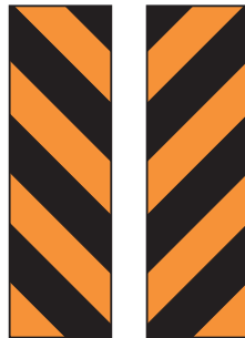
Hazard to left Hazard to right
