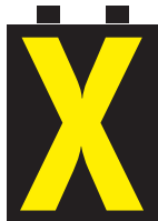
If flashing lane is for turning only; if solid direction of lane is changing
